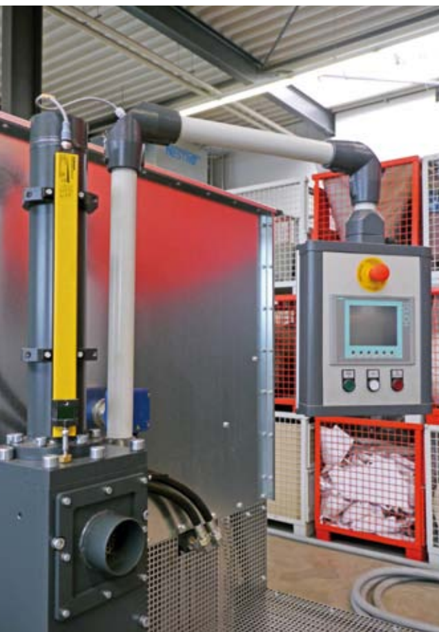
The analog signal of the LI sensor on the pre-compact is visualized directly on the control panel
