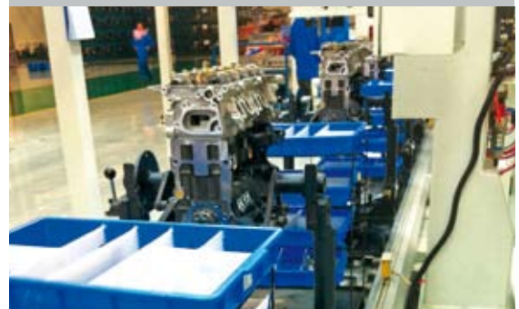
An automotive manufacturer in China is using Turck’s BL ident RFID system in a line to correctly coordinate the production of different engine versions. Page 30
