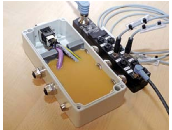
Indestructible: The customized I/O box is fully encapsulated and individually labeled by mechatec
