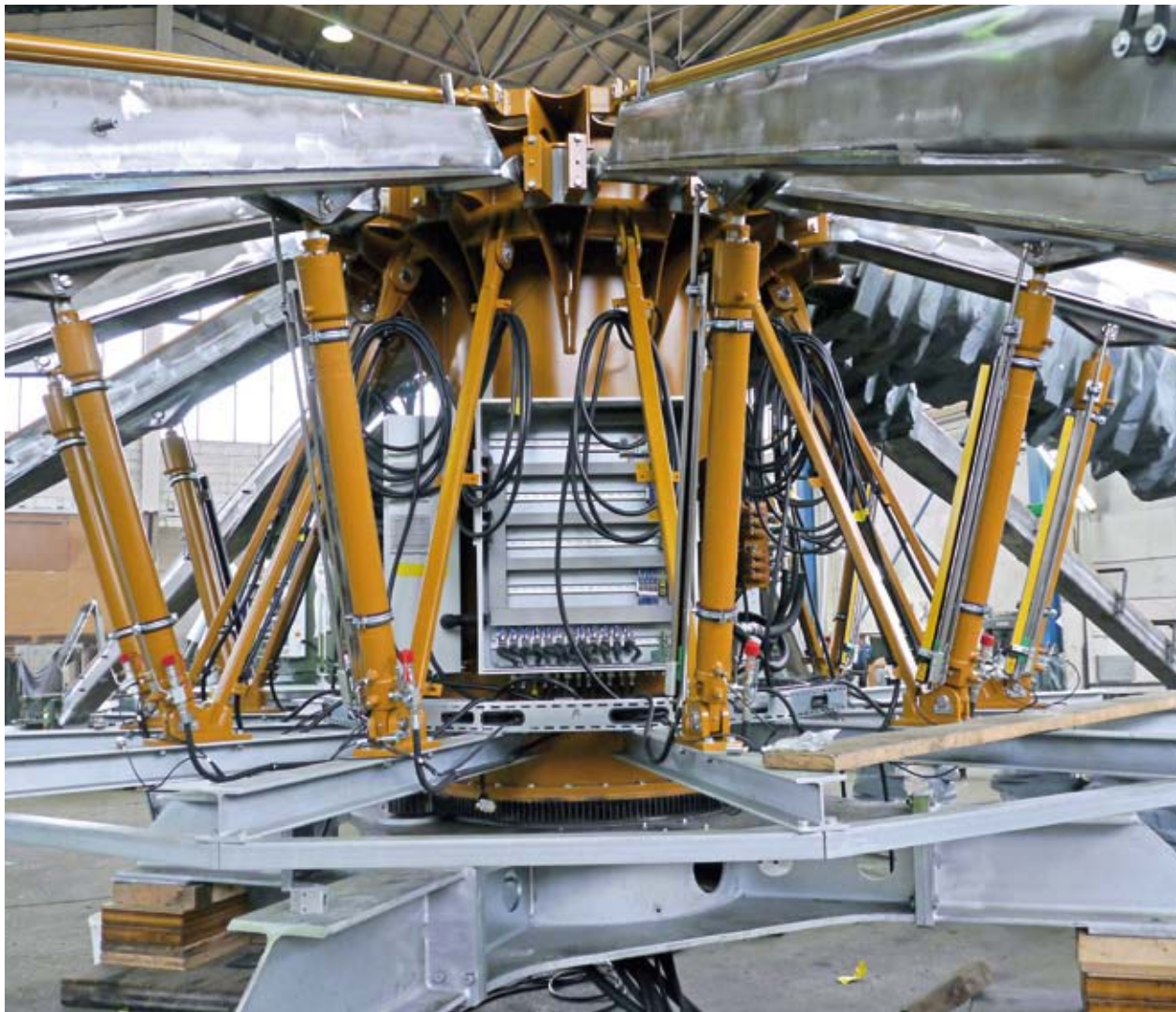
Instead of having to use five proximity switches for each hydraulic cylinder, a 1,000 mm linear position sensor from Turck now supplies the exact position of the arm
