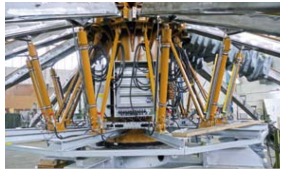
Zierer uses inductive linear position sensors from Turck to sense the horizontal position of the gondola arms on the Flying Fish roundabout ride. Page 22
